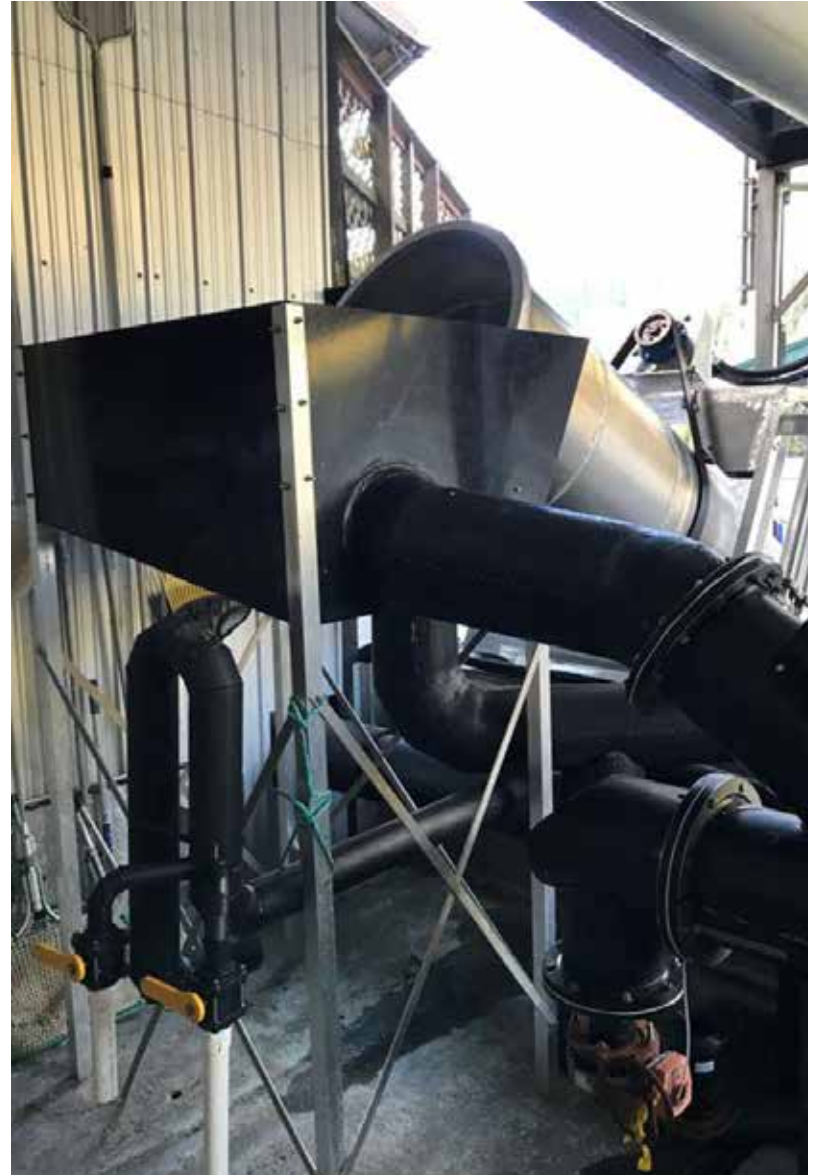
The new Archimedes screw gently lifts salmon to the processing equipment inside the hatchery facility. PHOTO BY ANNA TOLLFELDT
