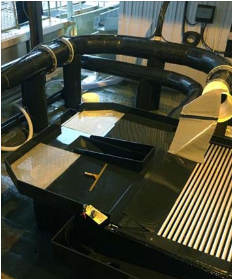
New equipment used in spawning salmon at Burnett Inlet Hatchery was custom-fabricated by the staff. The new process is gentler for egg sacs and more ergonomic for personnel. PHOTO BY ANNA TOLLFELDT
